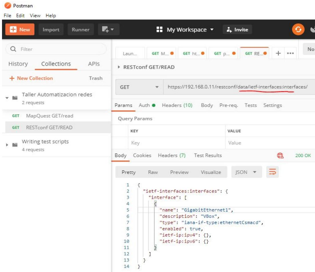
The screenshot shows the Postman interface with a RESTCONF GET request. The URL is `https://192.168.0.11/restconf/data/ietf-interfaces:interfaces/`. The response is a JSON object representing the configuration of the `ietf-interfaces:interfaces` container.
